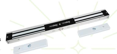
The NX-280DS Double Door magnetic lock is designed for use with wooden, glass, and steel doors with an opening angle of 90°. It has a maximum holding force of 280 kg (600 lbs) and can be used to control door opening and closing. The lock also features an indicator to show the door's status and supports signal output for testing the lock's status.
